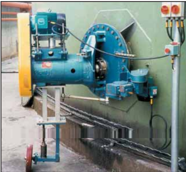
Swivel Angle Mixer ...with automatic actuator for continuous sweep of the tank floor in BS&W control applications. The version shown has a separate electric motor drive and castor wheel support. Also available with power take off drive and sling support from the wall tank.
