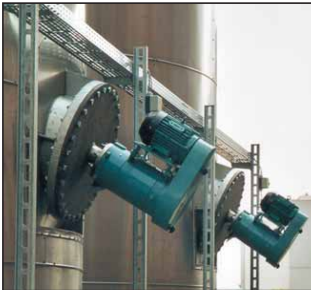
TM Series Mixer. Inclined installation - edible oil blending
