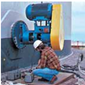
Swivel angle belt mixer undergoing site test as part of a continuing development program.
